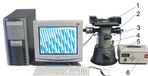
Fig. 1. Automated interference microscope. 1 – automated two-coordinate stage; 2 – support mirror on piezoelectric element; 3.5 – CCD cameras; 4 – microinterferometer; 6 – laser illuminator.
